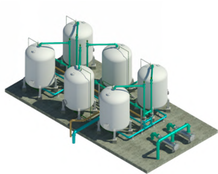
IX/FS TREATMENT (6: 12ft vessels)
